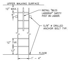
LADDER AND MOUNTING BOLTS SHALL BE CONSTRUCTED OF HOT DIPPED GALVANIZED STEEL. LOCATION TO BE DETERMINED IN FIELD.
